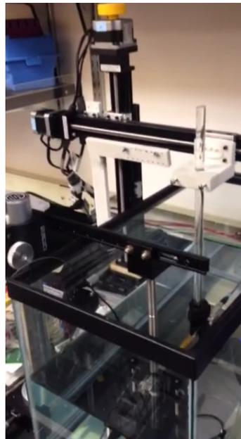
Figure A.5. Ultrasonic transducer and the hydrophone are immersed in a water tank and mounted on 3-axis linear, computer-controlled and manual stages, respectively, for XYZ beam scanning.
