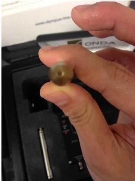
Figure A.6. 1 - 20 MHz broadband hybrid capsule hydrophone has an active area of  $400 \mu\text{m}$  at the tip, with  $160 \text{ nV/Pa}$  conversion. The hydrophone is attached to a switchable gain amplifier to increase its dynamic range.
