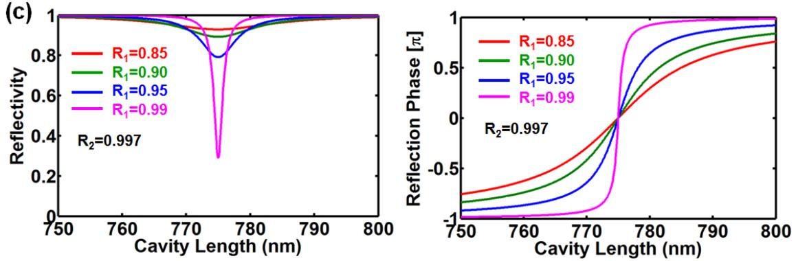
Figure 4.5 FP cavity reflectivity and reflection phase versus cavity length. The incident light wavelength is 1550 nm.  $R_1$  and  $R_2$  is the reflectivity of the top mirror and bottom mirror in power respectively.
