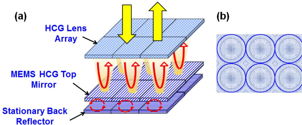
Figure 4.22 (a) Integrated optical phased array with HCG lens array. The effective filling factor of the phased array can be made to be 100%. (b) Layout of the HCG lens array.
