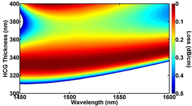
Figure 3.4 Loss contour plot against HCG thickness and operation wavelength, for a 1D slab HCG HCW with a 9  $\mu\text{m}$  waveguide height. The loss tolerance is very large over a wide range of HCG thickness and wavelength. The HCG period  $A$  and silicon grating bar width  $s$  is 1210 nm and 730 nm respectively.
