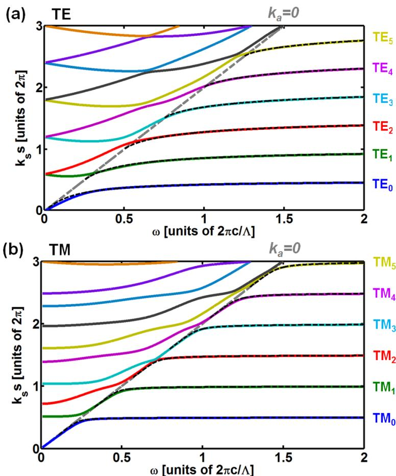
Figure 2.7  $\omega$ - $k_s s$  diagram of a waveguide array (solid) and a single slab waveguide (dash), for the same bar width  $s$  and index  $n_{bar}$ . This provides a physical intuition of the anti-crossing behaviors in the  $\omega$ - $\beta$  diagram. The  $k_a=0$  line is essentially the same as the air light line  $\beta=\omega/c$  in Figure 2.5. In this calculation,  $\eta=0.6$ ,  $n_{bar}=3.48$ ,  $\theta=50^\circ$ .
