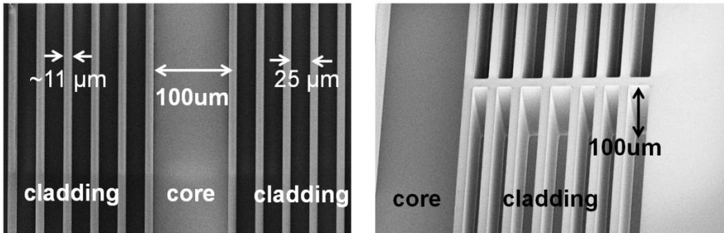
Figure 3.14 SEM image of the HCG-DBR hybrid HCW. The DBR structure is fabricated on an SOI wafer by deep etch Bosh process. Au will be subsequently deposited onto the exposed  $\text{SiO}_2$  layer. Another SOI wafer is patterned with HCG and would be placed on top of this wafer to form the 100  $\mu\text{m}$  by 100  $\mu\text{m}$  HCW.
