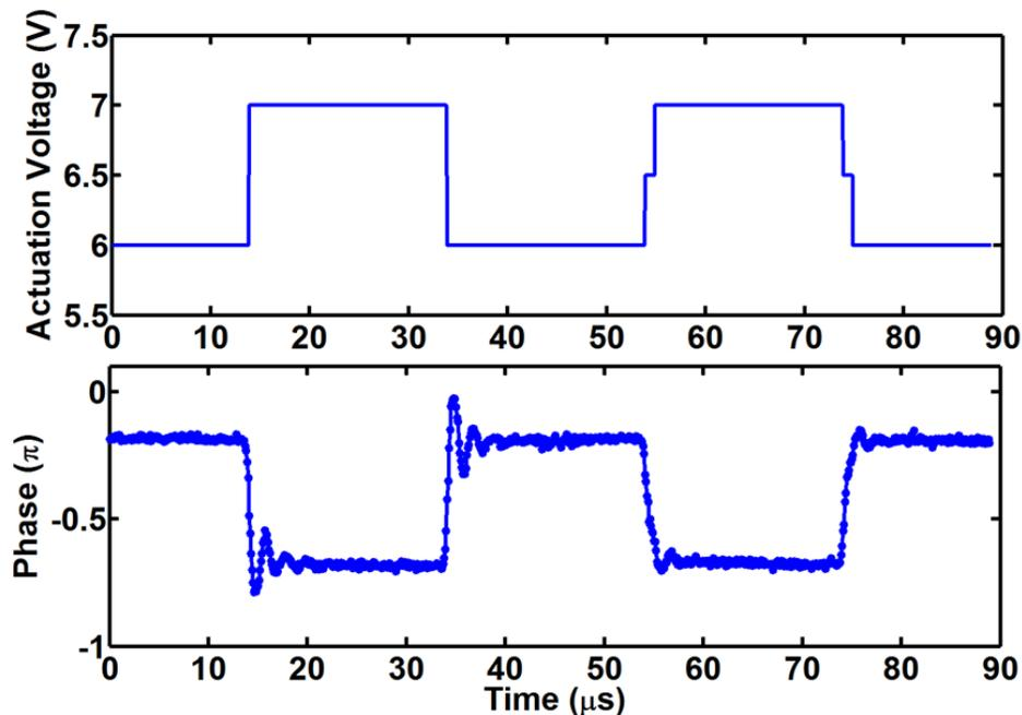
Figure 4.16 Comparison of the ringing between a one step and two step voltage control. In the two step voltage control case, the time interval between the two different step is  $1 \mu\text{s}$ , corresponding to half of the ringing period. The individual ringing from these two separate steps would have destructive interference, leading to an overall reduced ringing.
