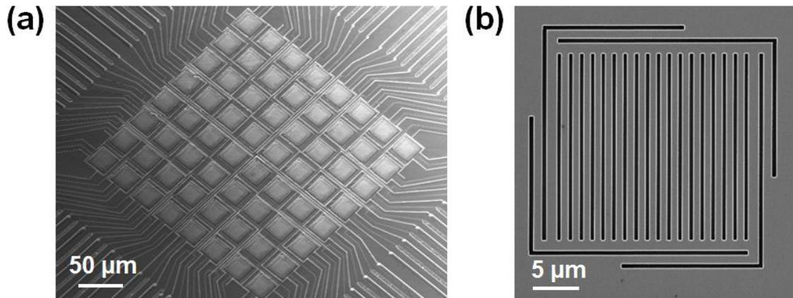
Figure 4.8 SEM image of an 8x8 optical phased array. Each pixel is an HCG-APF, which can be individually electrically addressed by the fanned-out metal contacts. The pitch of the HCG mirror is  $\sim 33.5 \mu\text{m}$ . (b) Zoom-in view of the HCG mirror in a single pixel. The HCG mirror size (without the MEMS) is  $20 \mu\text{m}$  by  $20 \mu\text{m}$ .
