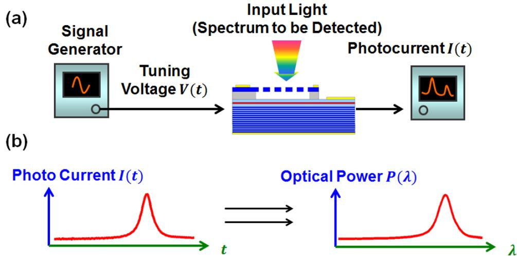
Figure 5.10 (a) Configuration of the optical spectrometer using the HCG swept-wavelength detector. A tuning voltage  $V(t)$  is applied to the HCG swept-wavelength detector, and the photocurrent  $I(t)$  is recorded versus time.  $I(t)$  is subsequently converted to  $P(\lambda)$ , shown in (b).
