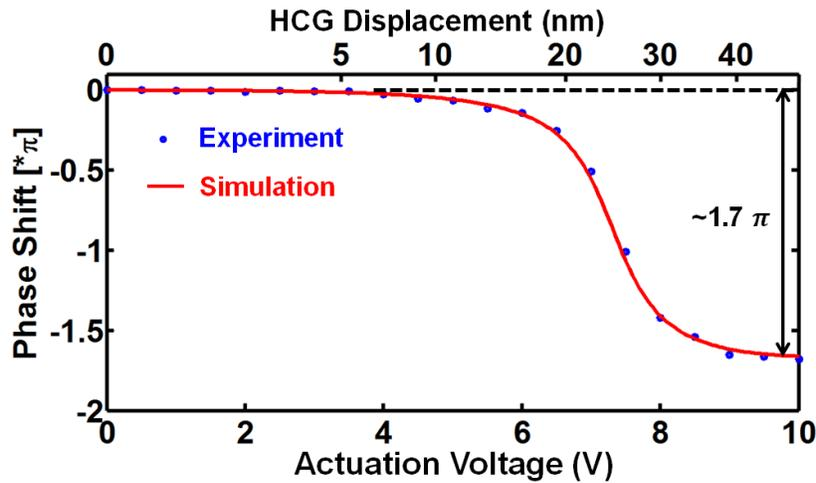
Figure 4.14 Reflection phase shift versus applied voltage on a single HCG-APF of the phased array.  $\sim 1.7 \pi$  phase shift is achieved within 10V actuation voltage range at a wavelength of 1556 nm; this corresponds to a displacement of  $\sim 50$  nm of the HCG. This APF design enables a small actuation distance for a large phase change. The experimental data (blue dots) are fitted with the simulation results with the DBR and HCG reflectivity of 0.9977 and 0.935 respectively (red curve).
