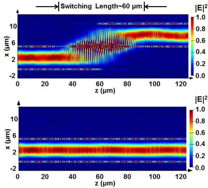
Figure 3.25 FDTD simulation of the HCG-HCW switch. The switching length is  $\sim 60 \mu\text{m}$ , and the refractive index change is  $-7 \times 10^{-3}$  at this switching region. The top panel shows the switch ON state, whereas the bottom shows the switch OFF state.
