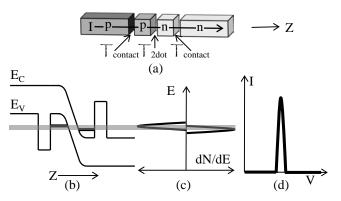
Fig. 5: The properties of a 0d-0d junction that is coupled to nanowire contacts are shown. (a) Schematic representation of the junction (b) Band diagram of the junction. (c) Tunneling only occurs at a single energy when the density of states in each dot is aligned. (d) The I-V curve resembles a delta function when the levels align.
