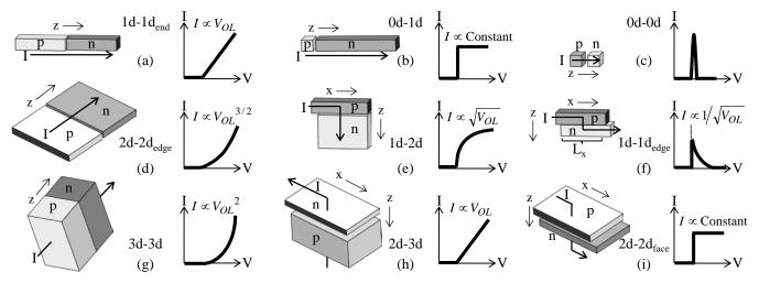
Fig. 2. We identify nine distinct dimensionality possibilities that can exist in pn junctions. Each of the different tunneling pn junction dimensionalities shown have different turn on characteristics as shown.
