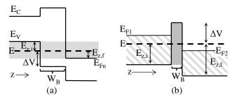
Fig. S2: (a) A rectangular band to band tunneling barrier. (b) A rectangular single band tunneling barrier.
