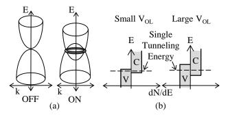
Fig. 6: Various characteristics of a  $2d-2d_{face}$  junction. (a) There is only a single tunneling energy because of the simultaneous conservation of energy and momentum. The energy versus wave vector paraboloids on each side of the junction only intersect at a single energy. (b) Even though the overlap of the density of states increases with increasing overlap voltage, there is only a single energy, indicated by the dotted line, at which the electrons tunnel.
