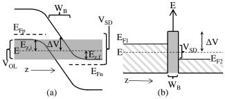
Fig. 3. (a) Energy band diagram for the tunnel pn junction showing that the relevant voltage is the overlap voltage and not the source drain voltage. (b) Energy band diagram for a typical 1d quantum of conductance showing that the relevant voltage is the source drain voltage.
