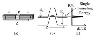
Fig. 4: (a) A 0d-1d junction converted into a more realistic 1d single electron transistor (SET) structure. The left nanowire can also be a p-type wire. (b) Band diagram corresponding to the SET. (c) All the current is concentrated around a single energy, which allows for a small overlap voltage  $V_{OL}$ , and thus a sharp turn on.
