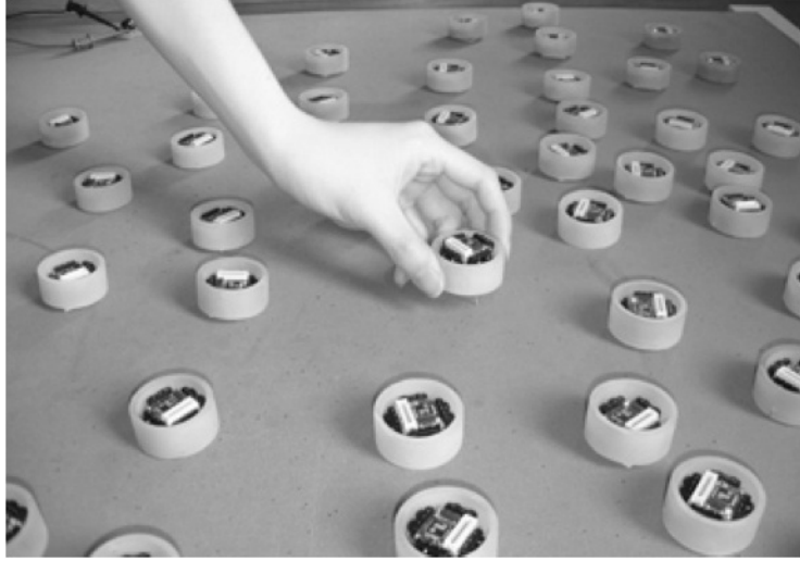
Figure 1.1. Pushpin nodes, a first implementation of the paintable computing concept [66]. Approximate node size is 3.24\text{cm}^2
