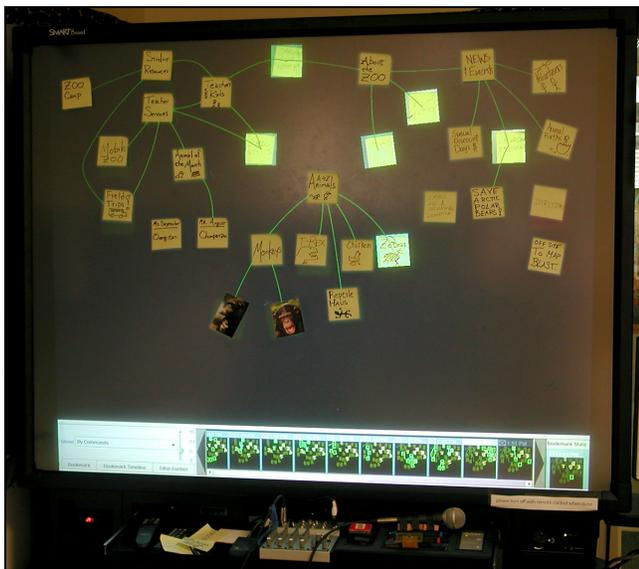
**Figure 1.** Users' view of history in the Designers' Outpost, a system for collaborative web design. Outpost runs on a touch sensitive SMART Board augmented with physical Post-it notes.
