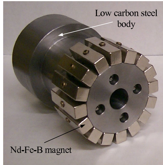
Figure 4.8: Fabricated power piston shown with the low carbon steel body and Nd-Fe-B permanent magnets attached to one end.
